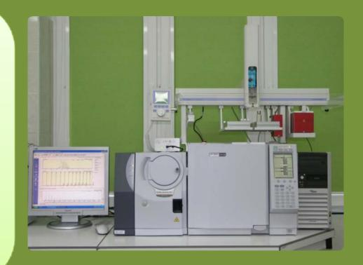
Hydrocarbon assays were made on a gas chromatograph with a Shimadzu mass detector (Gas Chromatograph Mass Spectrometer, GC-MS-QP 2010 Plus).
