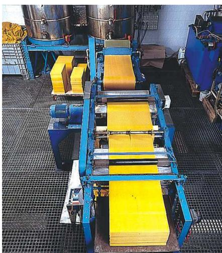
*Sheeting of beeswax* was the first method used in production of foundations. In a first stage wax sheets are produced and in a second the foundations are produced by calendering. The wax sheet is run through a foundation mill, which will print the foundations. Foundations produced by sheeting and milling is today the preferred method world-wide.
