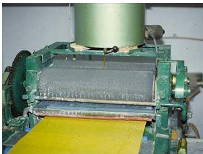
*Casting or Milling of wax* will produce foundations that are more brittle in the cold than milled sheets. Cast foundations are produced mainly by beekeepers, as this method is easy to perform in small beekeeping units.
